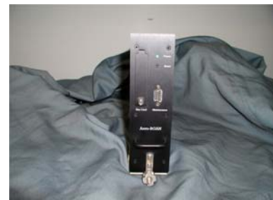
Thrane & Thrane's nye proof-of-concept Aero-BGAN terminal I en 2 MCU kabinet.
